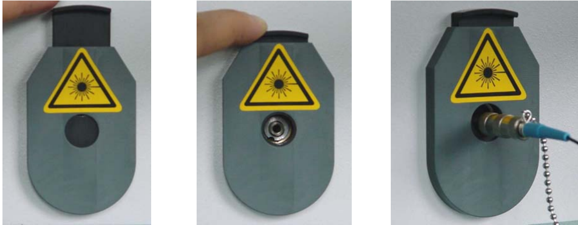
Fig. 13: Connecting the fiber
